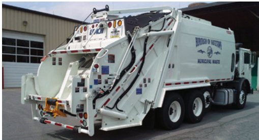
The Borough's first refuse truck outfitted with a cart tipper that can empty oversized receptacles is now in service.
