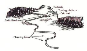
Climbing turns can be built on gentler slopes, usually not more than 15-20%. Switchbacks are needed on steeper slopes.
