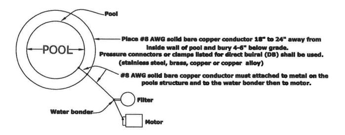
\*If pool pump motor is double insulated it shall not be bonded to this motor but instead shall be connected to the pool pump motor receptacle equipment grounding conductor (green).
